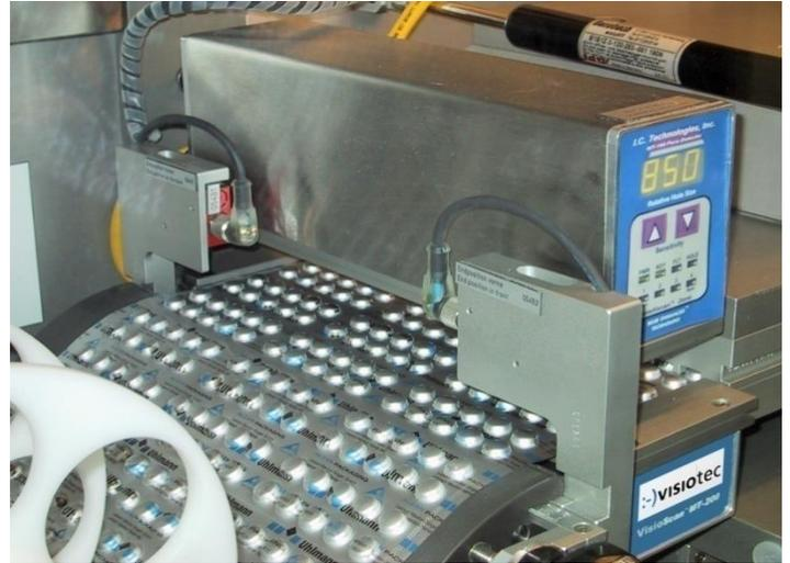
Pinhole inspection system VisioScan for aluminum forming material installed on an Uhlmann blister machine
